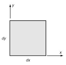
2-3. A two-dimensional problem of a rectangular bar stretched by uniform end loadings results in the following constant strain field:
